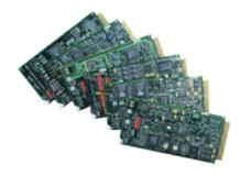
The Intraplex DA-191A and DA-191B asynchronous data modules each provide four RS-232 or RS-422 data interfaces.
