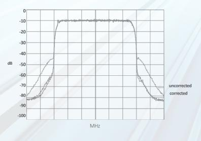
required to meet spectral emission compliance, but the filter itself introduces an undesired distortion. With linear pre-correction, the transmitted signal has optimal modulation performance so less equalization is required at the receiver.
