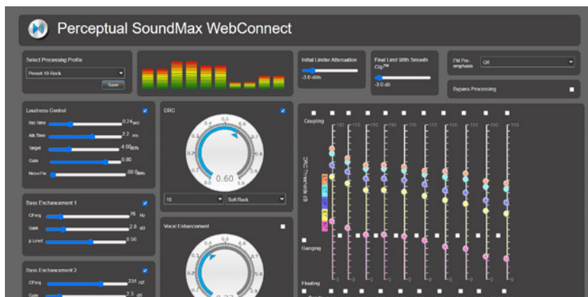
SoundMax WebConnect Web-based controller software runs on any browser, and can fine-tune and control the audio quality of SoundMax™ IP and generate new profiles.
