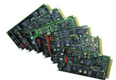
The Intraplex D-100 Infinity Data Module uses a unique rate justification method to provide transmission of any data rate from 0 bps to 1.968 Mbps, completely decoupled from network timing.
