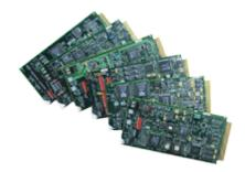
The Intraplex DA-91A is an Asynchronous Data Polling Channel Module designed for use in Intraplex ACS-160 and ACS-260 Series multiplexers. It provides one or two full duplex channels between an unlimited number of locations using a single 64 kbps DS0 time slot.
