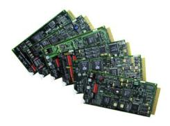
The GatesAir DS-562 is a serial data transport channel module that offers a flexible array of operating modes. It supports the transport of one or two channels of serial data.
