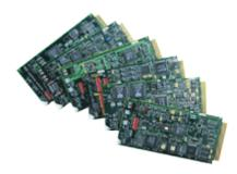
Intraplex 4-wire transmission-only voice frequency modules are available with PCM coding (64 kbps per channel) or ADPCM coding (32 kbps per channel).
