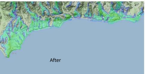
Coverage into the all-important Malibu area was virtually non-existent. With MaxxCasting, significant coverage is available. Even though this is fully FCC compliant, KPCC's coverage extended well past the contour, in this case (over water).
